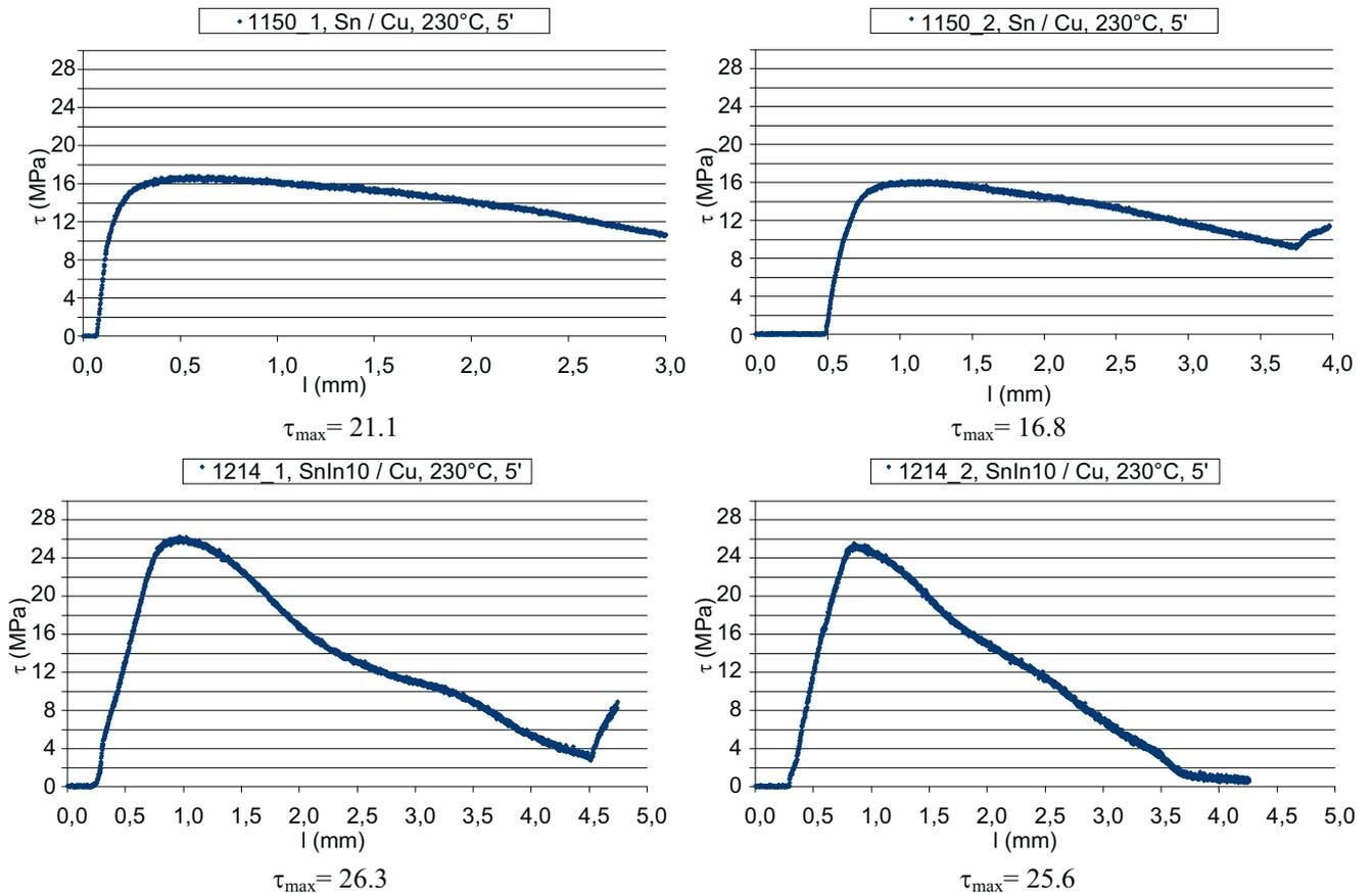
Fig. 2. Example-relationships between the maximum shear stress and a distance from the initial shear surface
