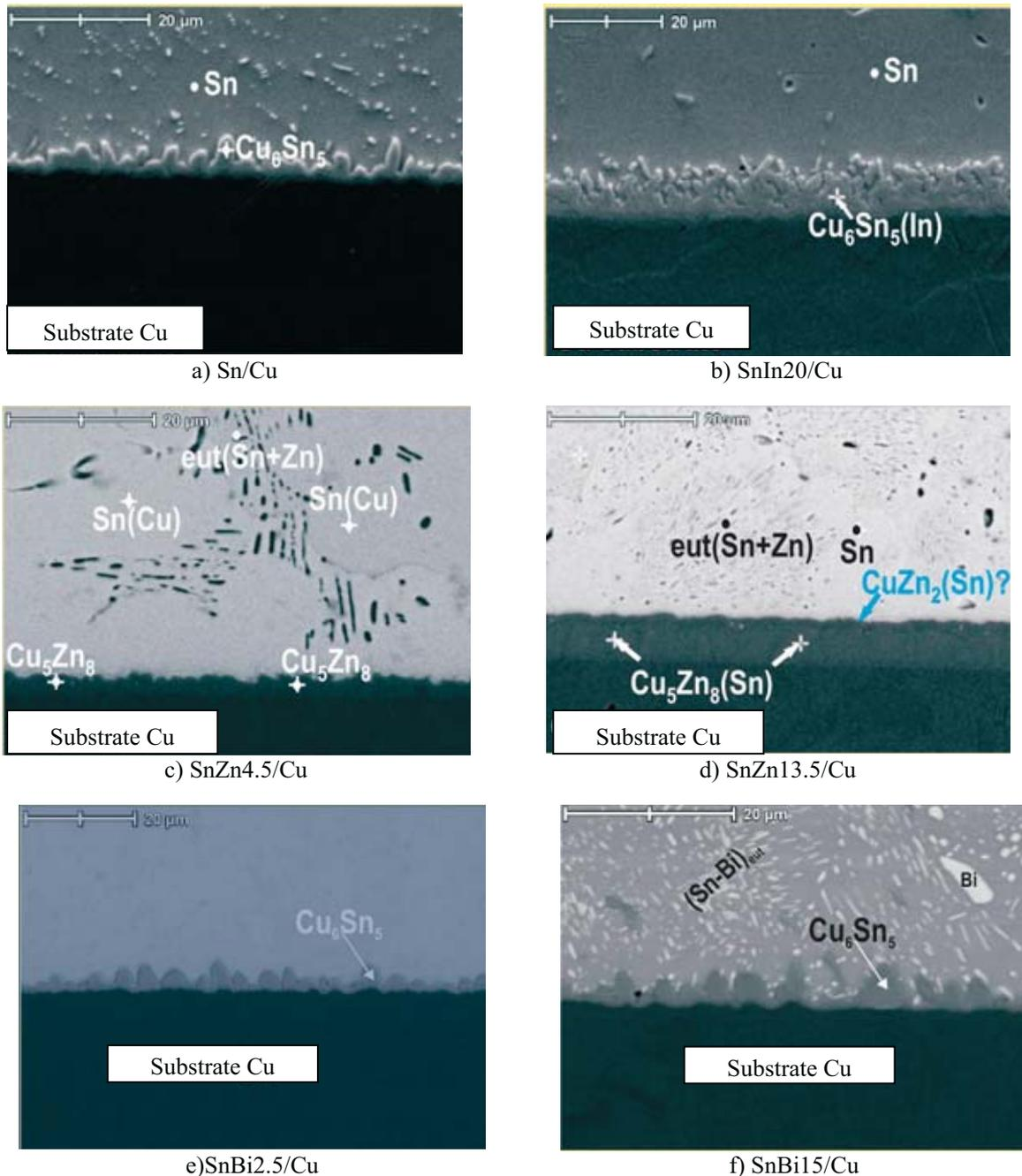
Fig. 3. Microstructures of investigated lead free solder/Cu substrate joints
