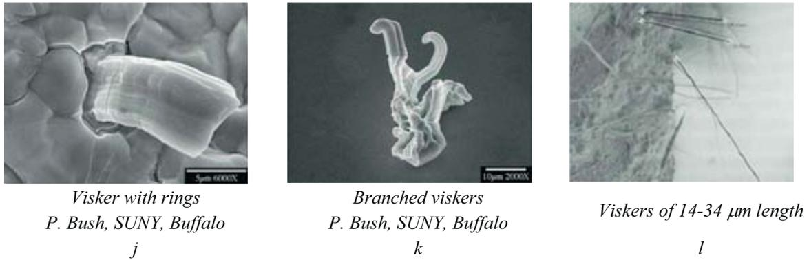
Fig. 1. Examples of the Sn viskers creation on substrate [5]
