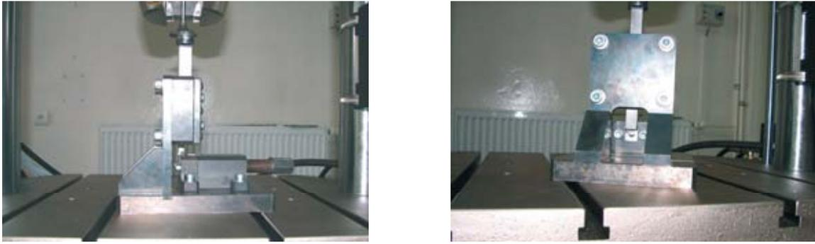
Fig. 1. Original equipment directly installed on the testing machine INSTRON 8874 for shear strength test
