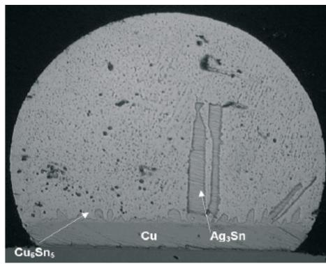
Fig. 2. Microstructure of solder drop on Cu substrate with phase identification [2]
